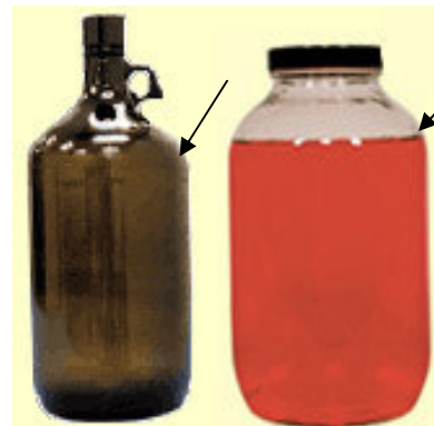
Do not fill past shoulder.
