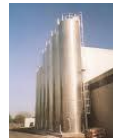
Silo – an outdoor, above ground tank which holds non-liquid materials
